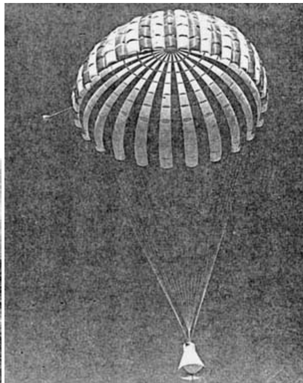
Figure 18. Main 63-foot ringsail parachute.
