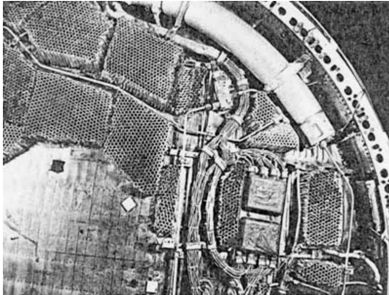
Figure 12. Honeycomb structure partially to absorb impact force.
